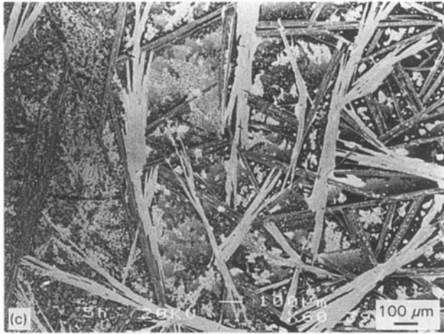
Figure 5 Back-scattered electron images of the surface of the films annealed at 890 °C for (a) 1 h, (b) 2 h, and (c) 5 h.
